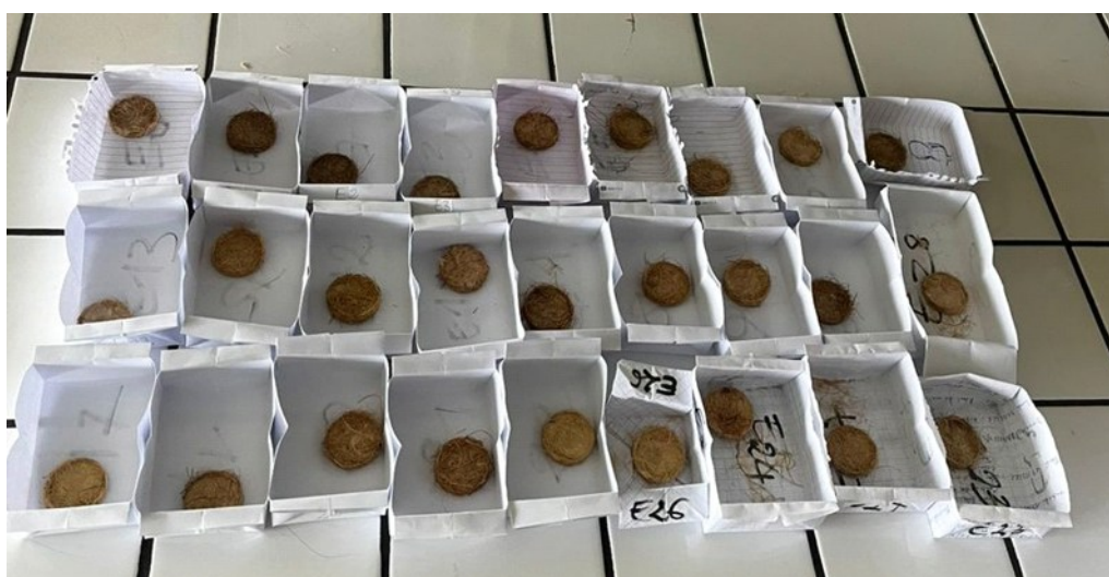
Fig. 9. Photographs of the samples of thermal insulation materials obtained
