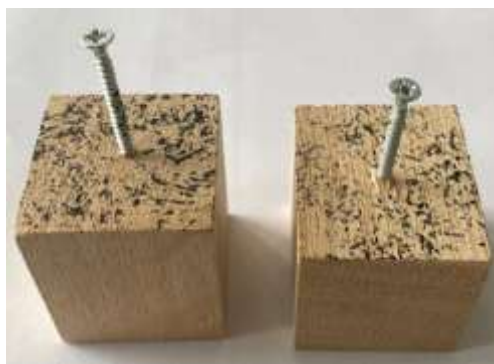
Fig. 2. View of the test specimen with a random speckle pattern applied for Digital Image Correlation (DIC) analysis and a wood screw installed
