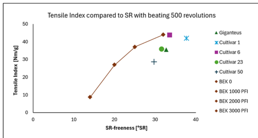
Fig. 5. Tensile index to Schopper-Riegler at 500 revolutions in the PFI mill for Miscanthus x giganteus and different Miscanthus cultivars, compared to bleached eucalyptus kraft refined at 0, 1000, 2000 and 3000 revolutions in the PFI mill.
