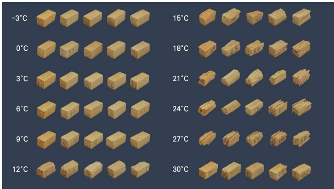
Fig. 3. Macro-photographic matrix of all replicated wood specimens after a one-week termite feeding assay
