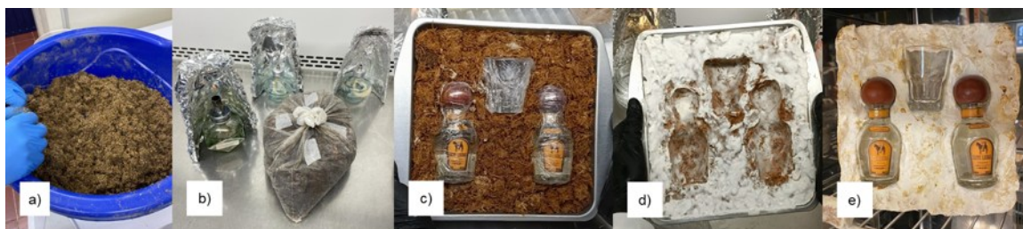
Fig. 1. Biofabrication process of Ganoderma composites: a) fiber hydration and sterilization, b) inoculation of the fiber with Ganoderma , c) mold filling, d) demolding, e) fungal inactivation and biomaterial drying
