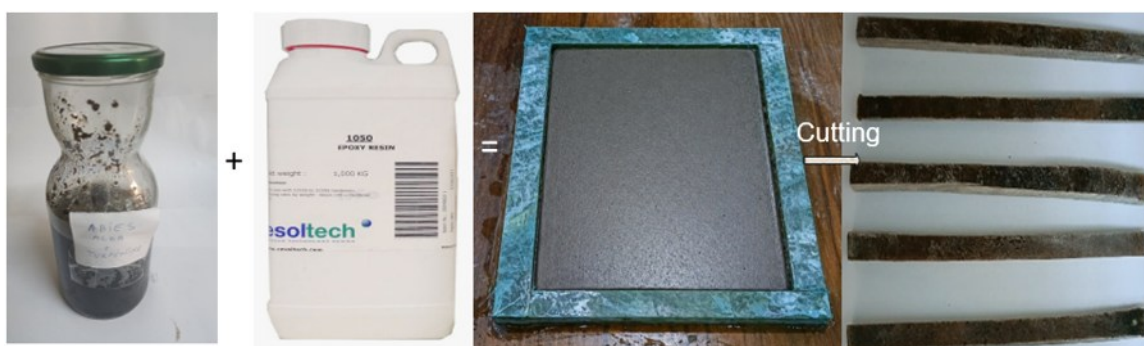
Fig. 2. Schematic representation of the process of combining natural and synthetic resins to obtain a solid material, along with the highlighting of specimens cut from the hybrid resin plate
