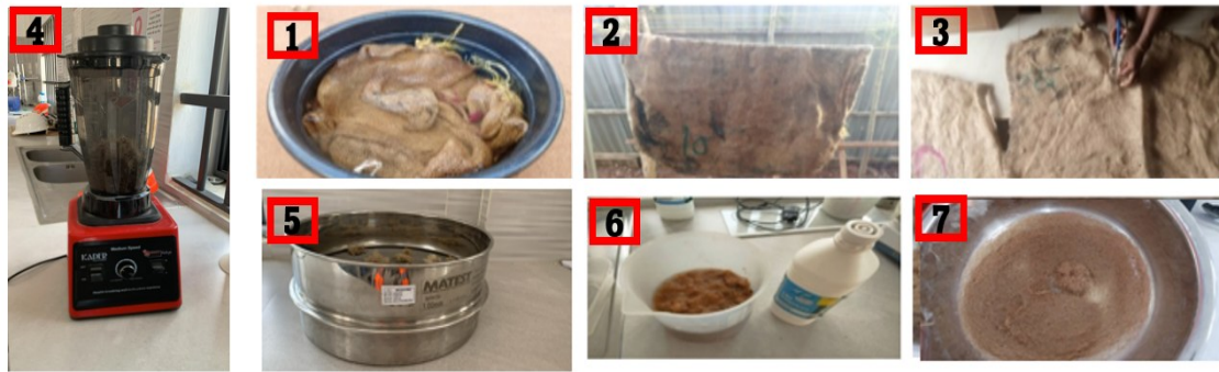
Fig. 1. Fiber extraction stages: 1: Washing the bags with potable water; 2: Air drying; 3: Defibration of jute bags; 4: Grinding the cut jute fibers using a mill; 5: Sieving the jute fibers through a 1 mm sieve; 6: Purifying the fibers using demineralized water; 7: After rinsing, the fibers underwent air-drying in a controlled laboratory environment ( 23 \pm 2^\circ\text{C} , 50 \pm 5\% RH) until a constant mass was achieved.
