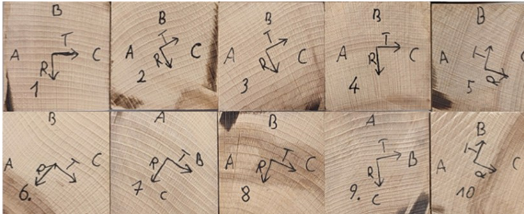
Fig. 1. Sample designation indicating the orientation relatively to the fibres tangential T, or radial R direction of processing
