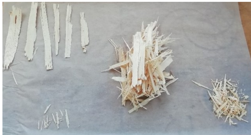
Fig. 1. Two fractions of strands that were used for LSL productions
