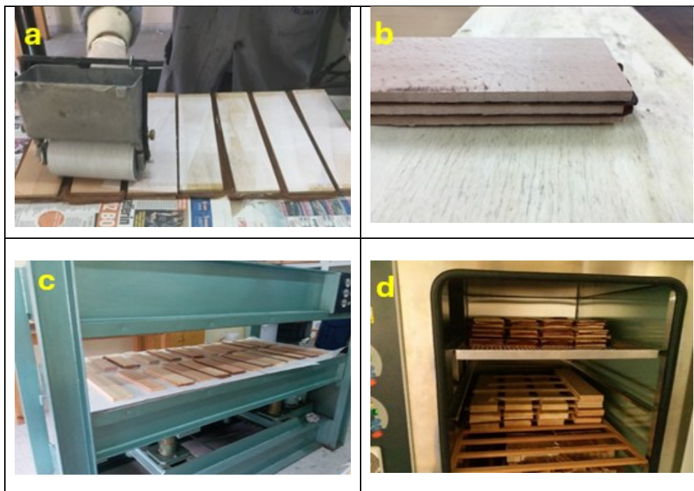
Fig. 3. Production stages of BC-reinforced laminated wood materials: (a) adhesive application, (b) layering, (c) pressing, and (d) conditioning. Reproduced from Part 1 (Budakçı et al. 2025) to ensure experimental consistency
