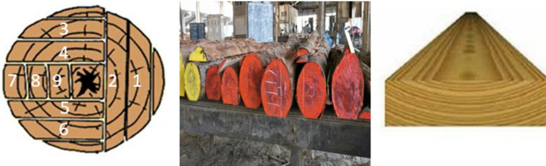
Fig. 3. Back-sawing pattern of the logs
