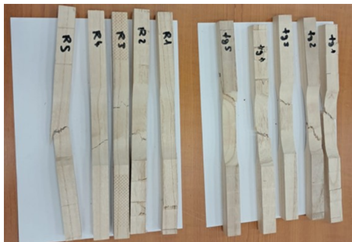
Fig. 13. The samples for tensile strength parallel to the wooden fibers
