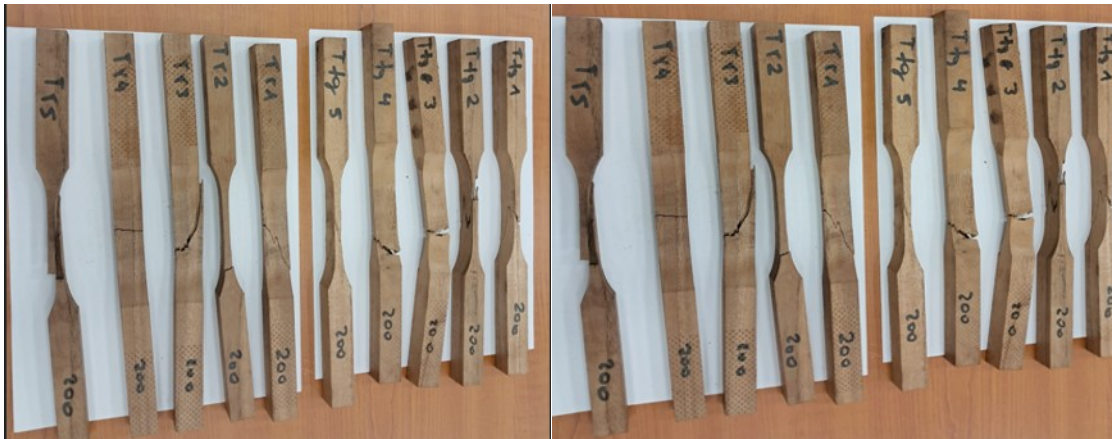
Fig. 4. Tensile strength parallel to the grain of the samples
