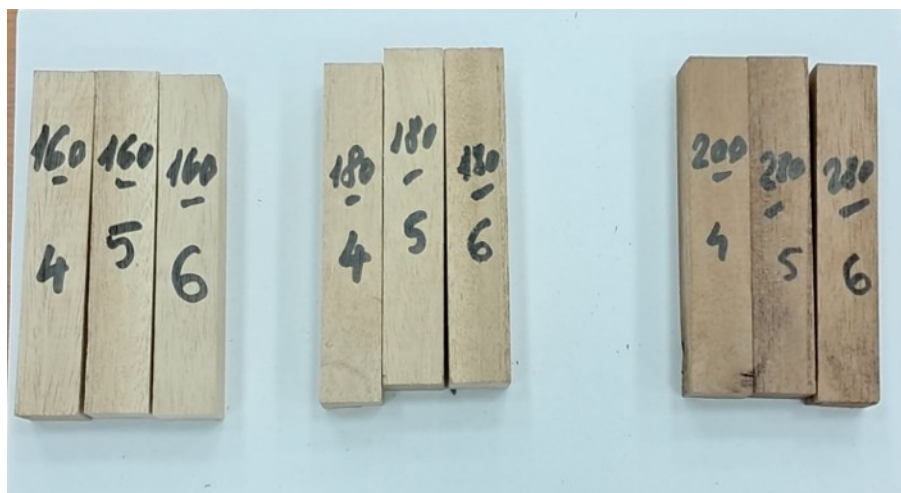
Fig. 2. Samples of Paulownia tomentosa torrefied at 160^\circ\text{C} , 180^\circ\text{C} , and 200^\circ\text{C}
