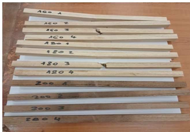
Fig. 3. Torrefied bending testing specimens after testing
