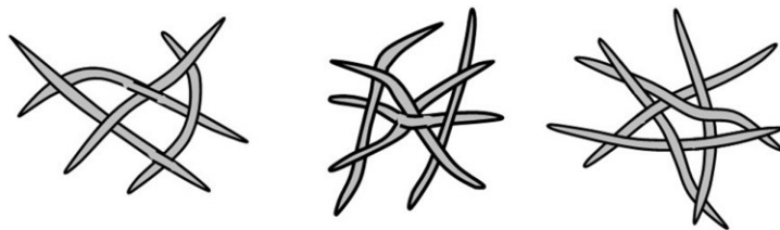
Fig. 8. Depiction of some simple fiber flocs in which just a few fibers may be held together by a combination of fiber-to-fiber friction and elastic forces of straightening after fibers have become momentarily bent by eddies of flow (examples redrawn based on originals by Parker (1972))
