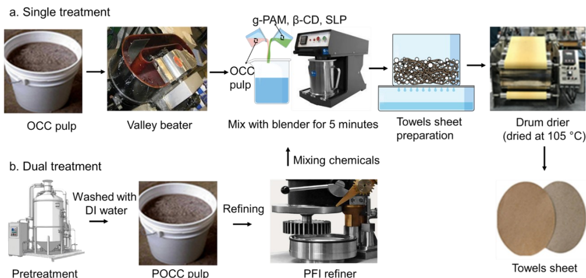
Fig. 2. Schematic illustration of single- and dual-stage treatment strategies for paper towel sheets preparation from recycled fibers. (a) Single-stage treatment involves refining OCC pulp followed by addition of g-PAM, \beta -CD, or soy lecithin (SLP), paper towel sheets formation, and drum drying. (b) Dual-stage treatment incorporates autohydrolysis pretreatment to produce POCC pulp, followed by PFI refining, chemical addition, paper towel sheets preparation, and drying.
