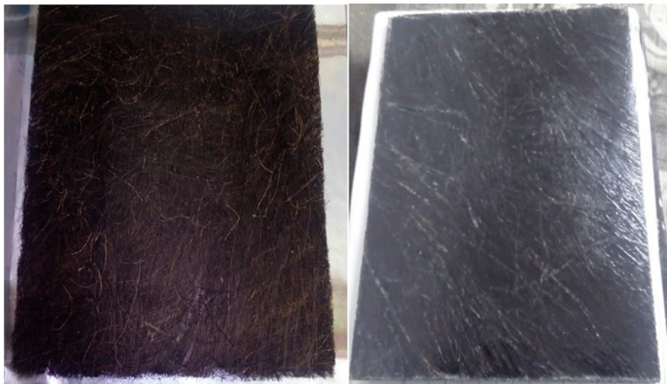
Fig. 2. The sugar palm fibers prepared for fabrication and the fabricated composite plate
