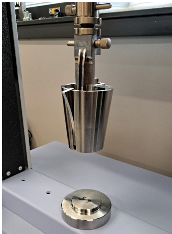
Fig. 2. Finished seal strength analysis device attached to the universal tester
