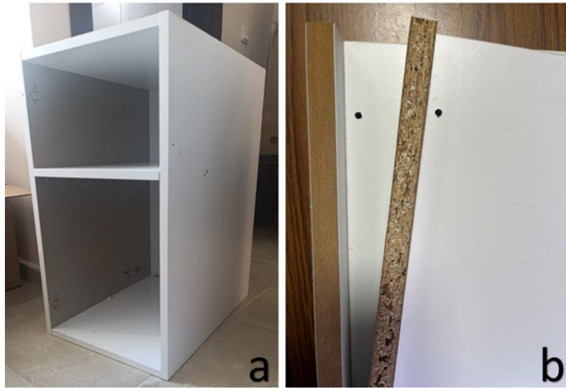
Fig. 1. Representative MDF and PB shelves used in the experiments, illustrating cabinet dimensions and side-view configurations of the shelf specimens
