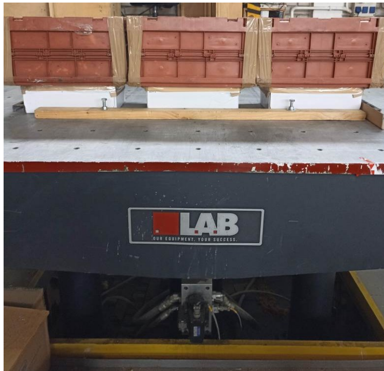
Fig. 5. Random vibration table test stand – L.A.B. Type HV88 from L.A.B. (Itasca, USA)
