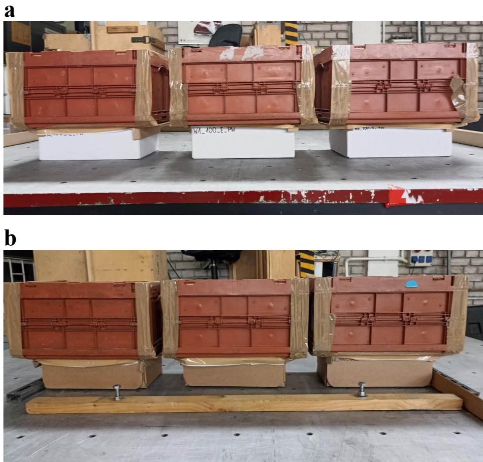
Fig. 7. Photos of the boxes during vertical vibration tests with equivalent load: (a) W1 samples and (b) W2 samples
