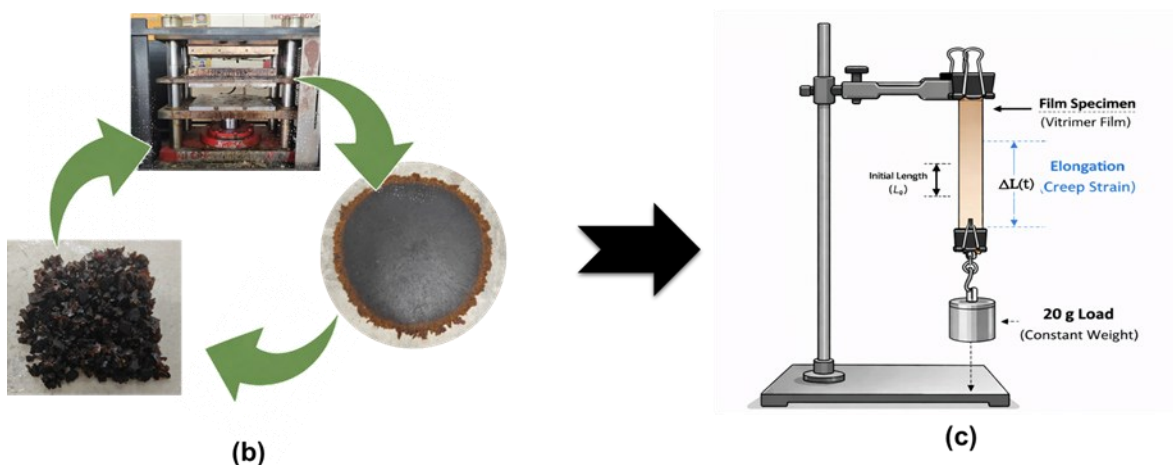
Fig. 1. (b) Reprocessing of vitrimer composites; (c) Schematic of creep-recovery test
