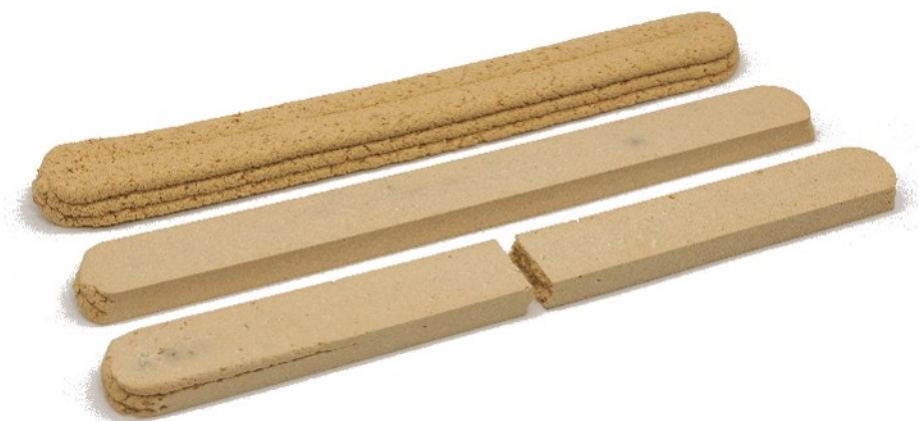
Fig. 5. Printed and sanded specimens for flexural strength measurement (reprinted with permission from Emerald Group Publishing, Rosenthal et al. 2023)
