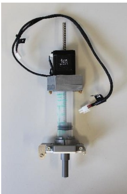
Fig. 4. Modified paste extruder with stepper motor, cartridge, nozzle and connecting elements (reprinted with permission from Emerald Group Publishing, Rosenthal et al. 2023)
