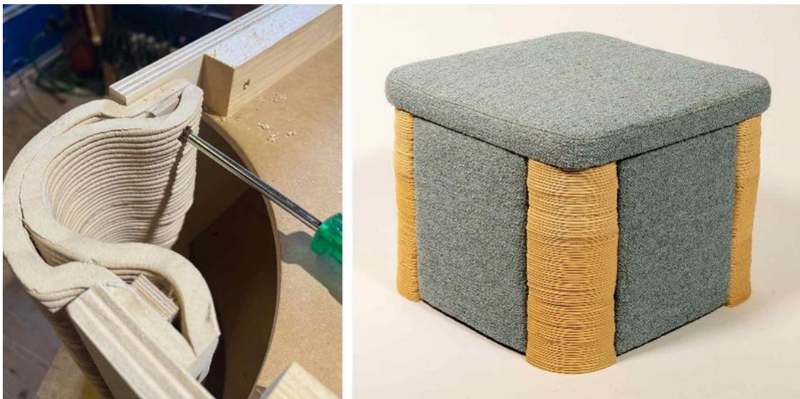
Fig. 1. Hybrid upholstered stool constructed from round corner elements made from additively manufactured wood-based paste (Bodenschatz and Rosenthal 2024) and traditional wood panel materials (U. Bodenschatz)
