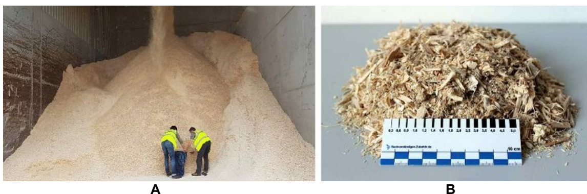
Fig. 2. Sampling at the HS Timber Productions wood particle storage facility (A) and dried particle material (B)
