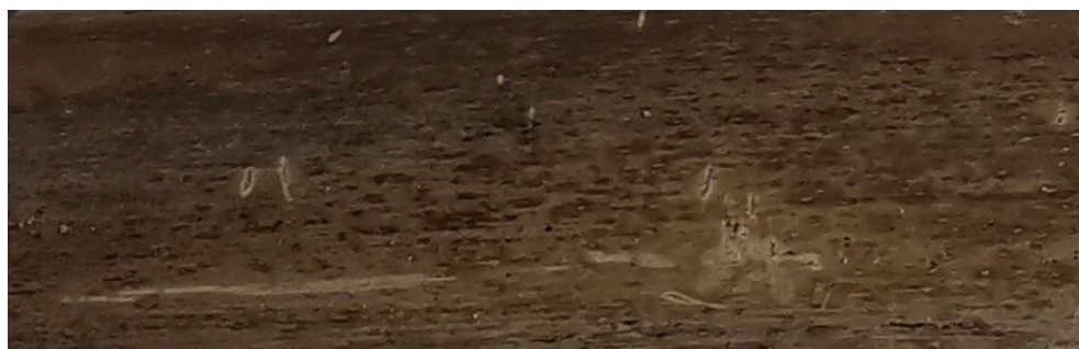
Fig. 5. Surface of bamboo after HVE treatment
