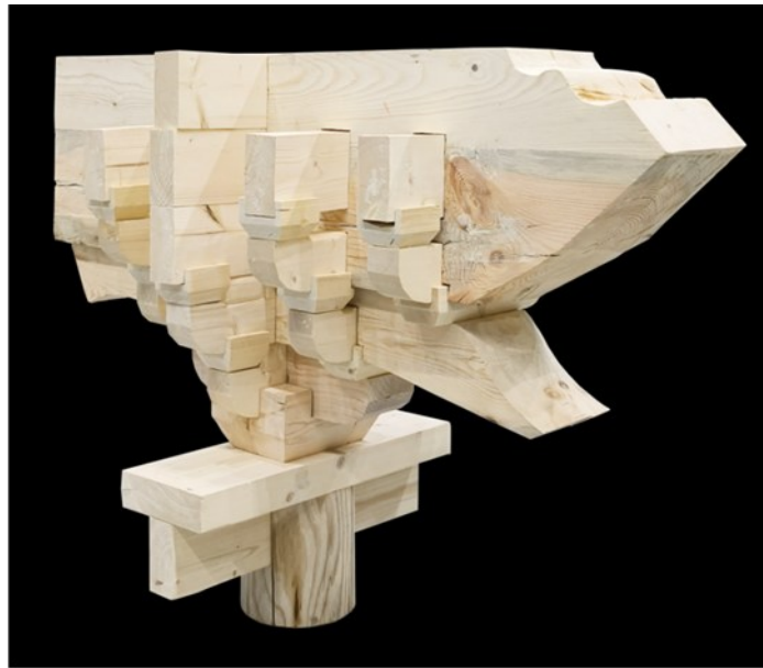
Fig. 3. Structural test model of bucket arch in Qing Dynasty
