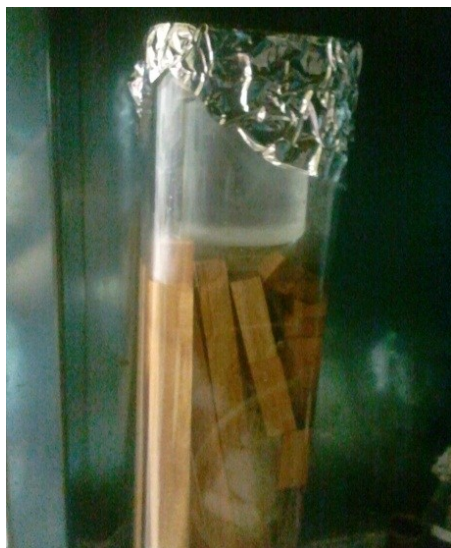
Fig. 1. Beech wood samples impregnation into the acetic anhydride
