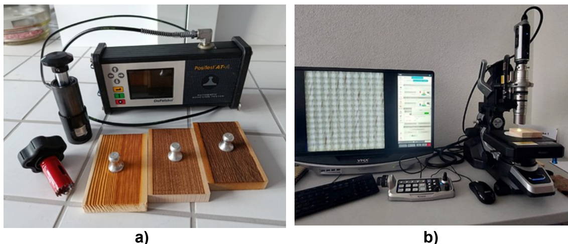
Fig. 3. The adhesion of the coating films was evaluated using the pull-off test: a) the PosiTest AT-A Pull-off Adhesion Tester measures adhesion of coatings; and b) the digital microscope Keyence VHX-7000
