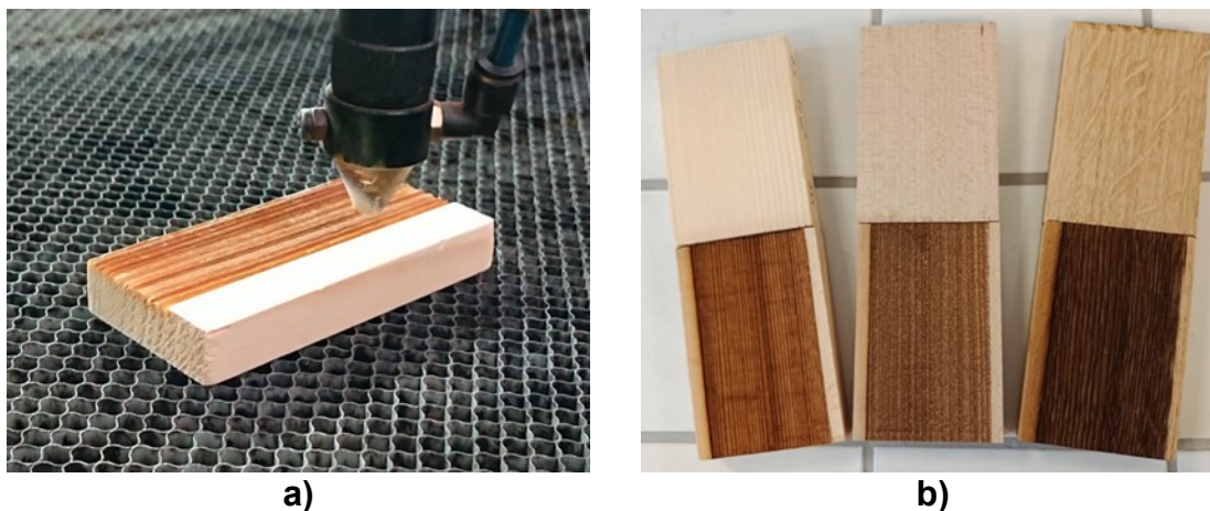
Fig. 1. The laser engraving: a) The sample positioned under the lens of a CO 2 laser system; and b) the laser-treated three wood species (spruce, beech and oak wood)
