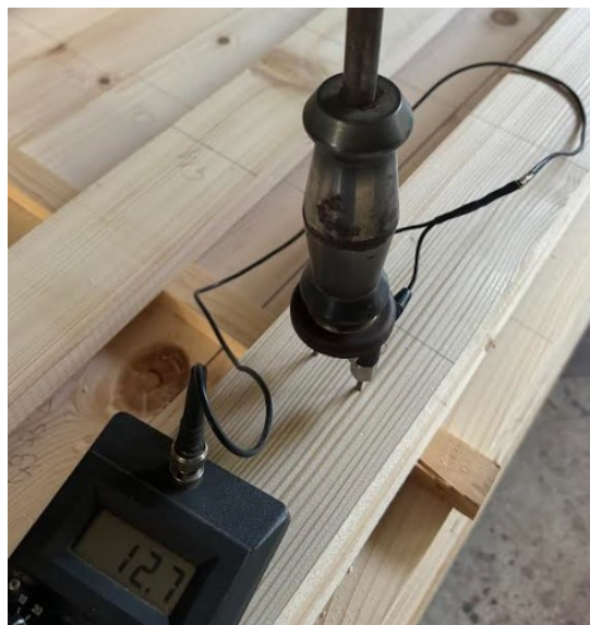
Fig. 3. Measuring moisture content using electrical resistance method (Hydrometer HT 65, GANN, Germany)
