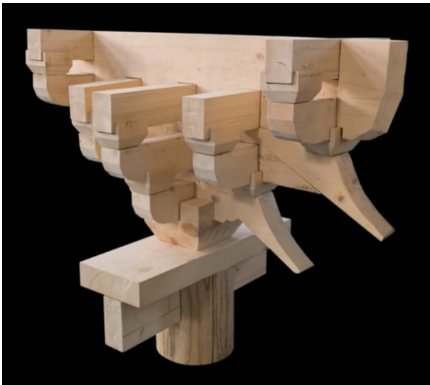
Fig. 3. Perspective view of the Yuan Dynasty bracket structure experimental model
