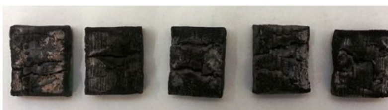
Fig. 2. Post-exposure photographs of spruce samples after radiant heat testing, showing differences in char morphology and surface integrity
