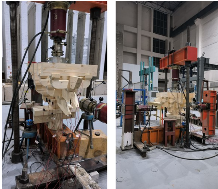
Fig. 7. Experimental loading apparatus for the 1:5 scaled bracket model
