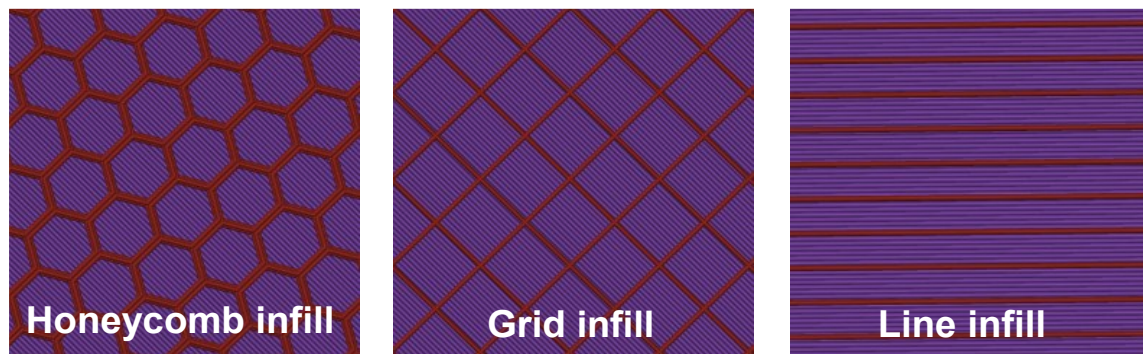
Fig. 2. Schematic diagram of infill structures
