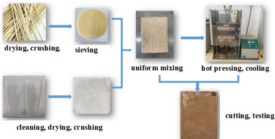
Fig. 1. Preparation process of waste PP/BF composites
