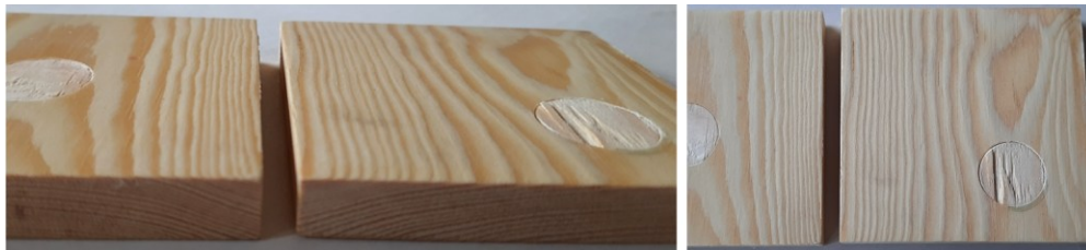
Fig. 2. Irregular (wavy) surface formed after varnishing in densified pine specimens
