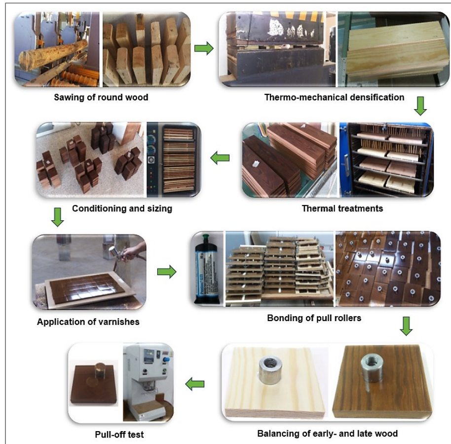
Fig. 3. Experimental process of the study
