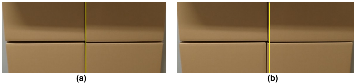
Fig. 9. Arrangement of boxes in columns: a) the axes of symmetry of the corners of the boxes coincide, b) the axes of symmetry of the corners are shifted relative to each other
