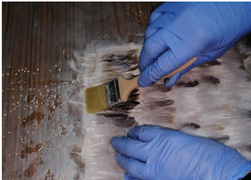
Fig. 2. An example of applying resin to the lamina using hand lay-up
