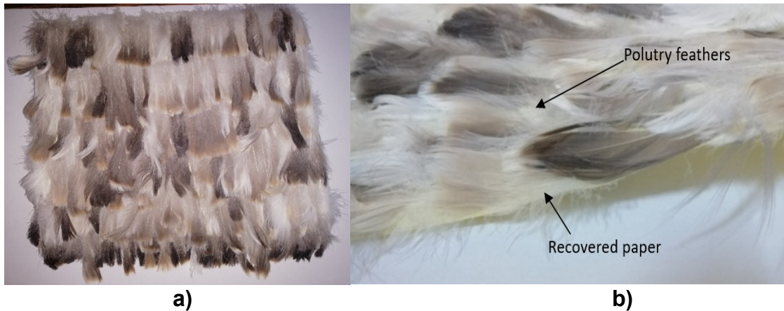
Fig. 1. a. An example of a lamina made of poultry feathers and recovered paper; b. detail highlighting the poultry feathers and recovered paper
