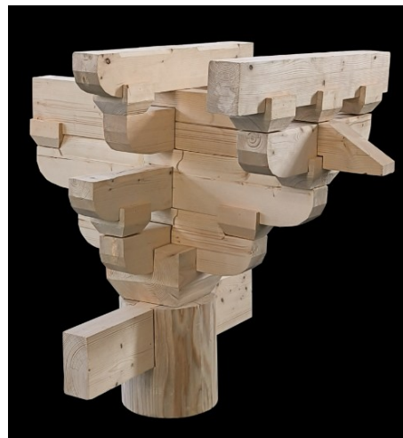
Fig. 3. The perspective view of 'Five-tier Outer Eave Column-head Dougong Bracket' test model of the Dule Temple Gate
