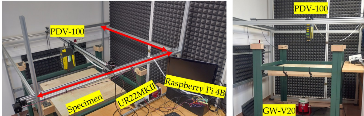
Fig. 3. The setup used for experimental modal analysis. The red arrows indicate the movement of vibrometer at the testing frame.
