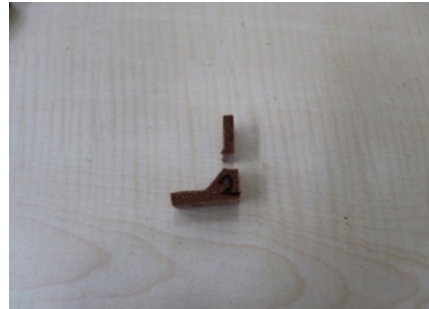
Fig. 11. Example of deformation after diagonal compression test on wood polymer LSBs
