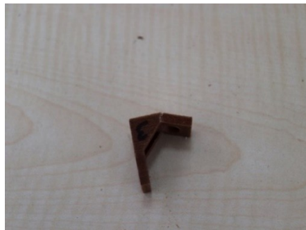
Fig. 13. Example of deformation after diagonal tensile test on wood polymer LSBs
