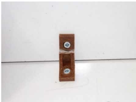
Fig. 12. Example of deformation after diagonal tensile test in CJWLSBs
