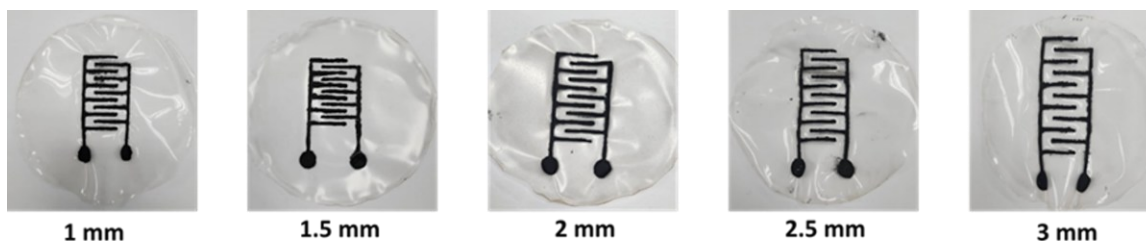
Fig. 1. Interdigitated electrode with different electrode finger spacing
