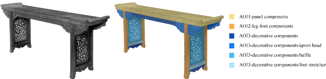
Fig. 3. AOI division of the experimental samples: AOI-1: Panel components; AOI-2: leg-foot components; AOI-3: decorative components (with sample GA2)
