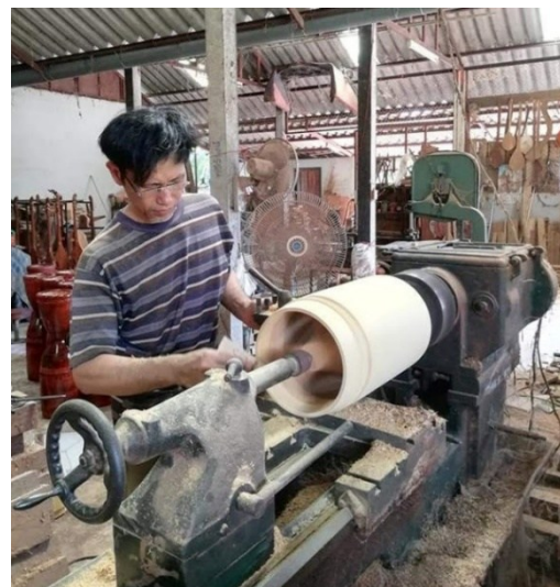
Fig. 15b. Turning wood to shape the drum
