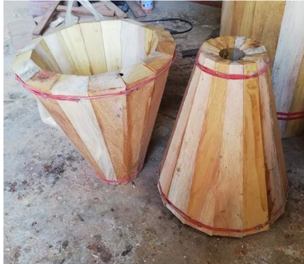
Fig. 14. Glue and glue the wood together in pairs, a total of eight pairs
