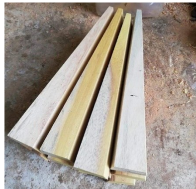
Fig. 13b. Saw the wood into at 14°
