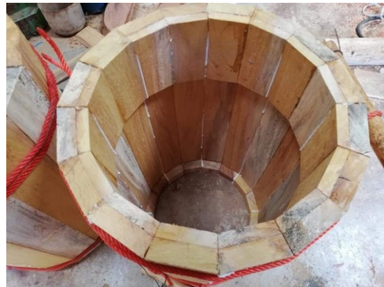
Fig. 10a. Model for the holding angle upper section Fig. 10b. Glue all 16 pieces of wood together.
