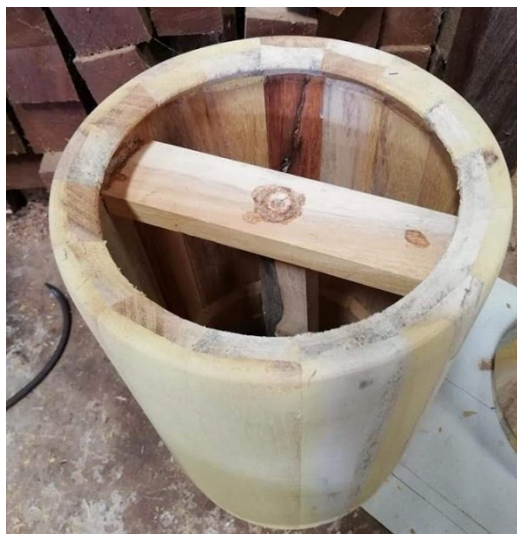
Fig. 15a. Use a stick to support the drum
