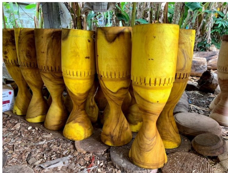
Fig. 2a. The Isan long drum has been turned and coated with urethane
