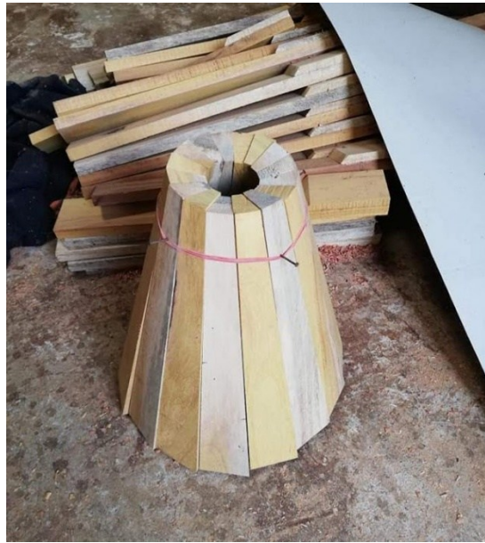
Fig. 12c. Glue the wood together and tie it with rope for about 2 days
