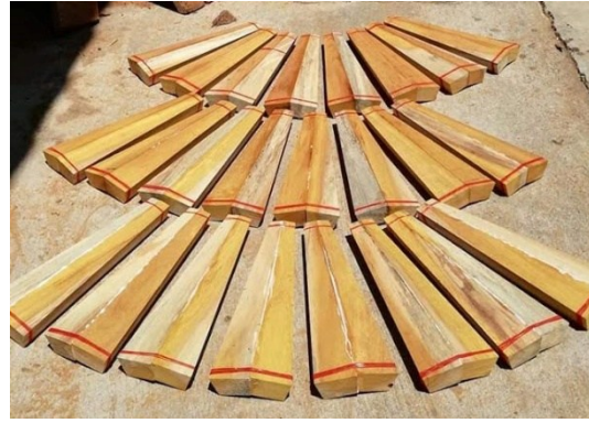
Fig. 12b. Glue the wood together into 8 pairs
