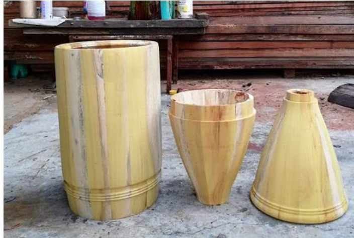
Fig. 16a. All three drum parts have been machined
