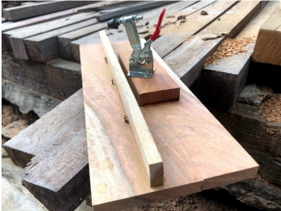
Fig. 10a. Model for the holding angle upper section Fig. 10b. Glue all 16 pieces of wood together.
