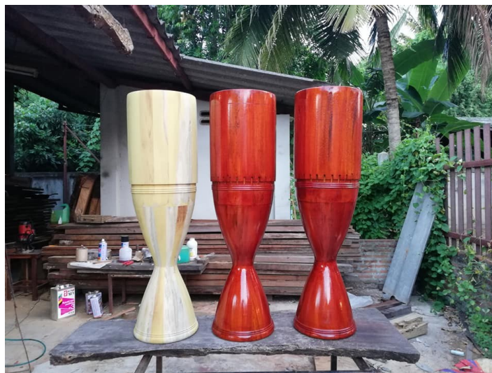
Fig. 16b. Assemble the three drum pieces
