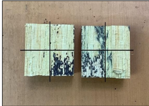
Fig. 3. Surface failure for laran glulam sample for initial condition with failure at 90%
