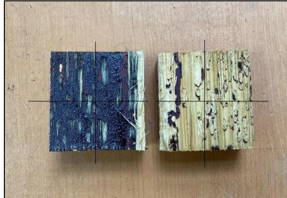
Fig. 4. Surface failure for laran glulam sample for water-soak (treatment 1) with failure at 50%
