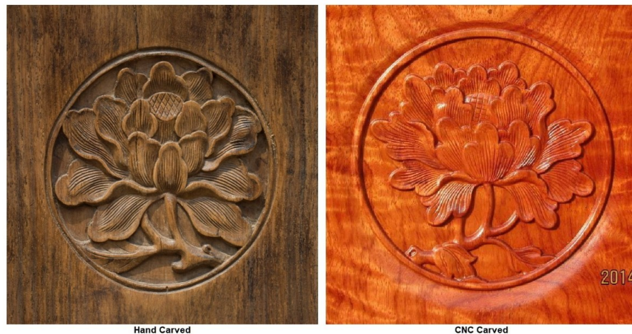
Fig. 5. Comparison between hand and CNC carving
