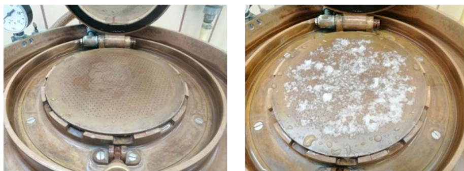
Fig. 3. Residues after desintegration (20 min) of paper (left) and ACC with a dissolution time of 30 s (right) on a Brecht-Holl-fractionator
