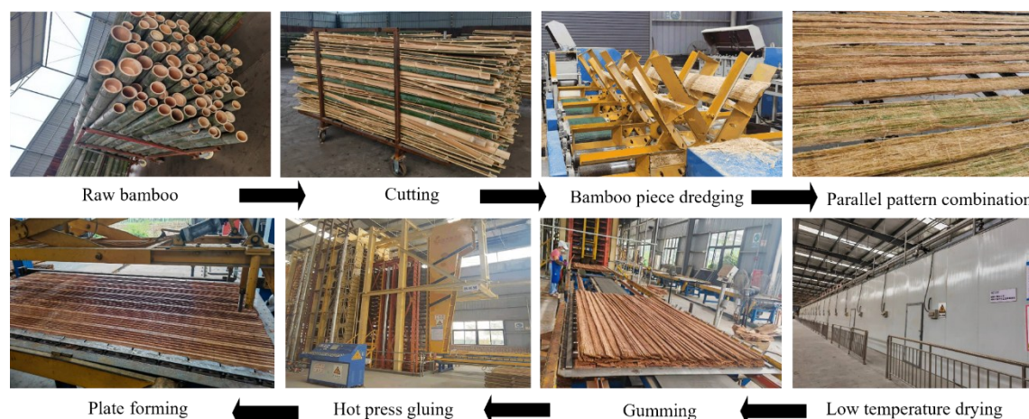
Fig. 1. Bamboo scrimber production process
