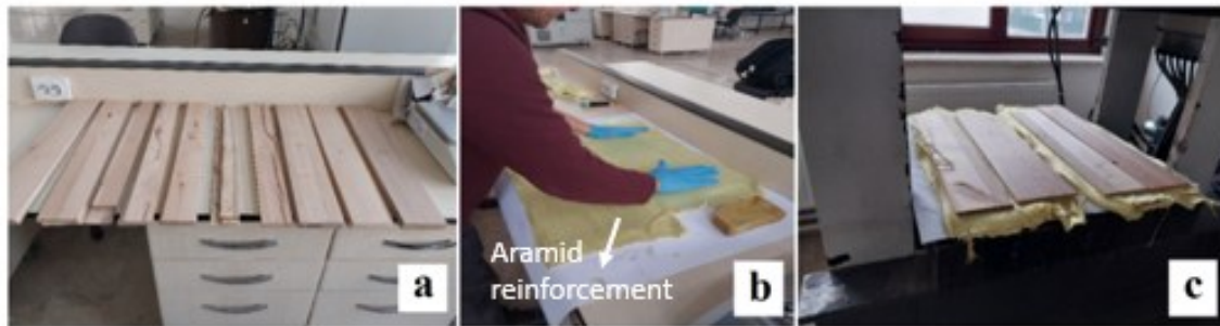
Fig. 2. (a) Cutting the wood, (b) Placement of the aramid reinforcement between layers (only for aramid-reinforced specimens), and (c) Placement of the upper layer
