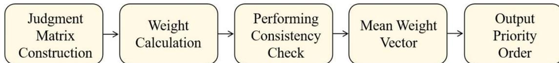
**Fig. 2.** Evaluation Indicator Weighting Flowchart
