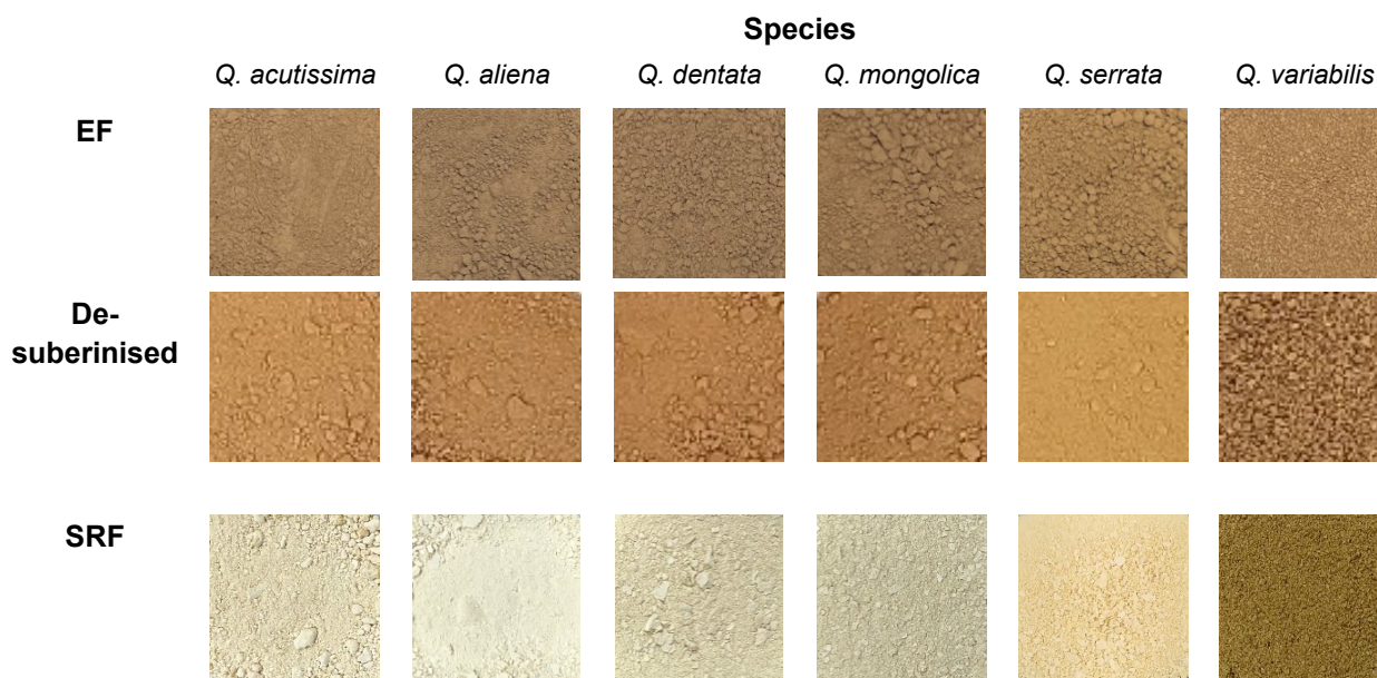
Fig. 2. Qualitative color results of extract-free (EF), desuberinised material, and Suberin-rich fraction (SRF) of six Korean Quercus species (EF = SRF + lignin + carbohydrate; Desuberinised = lignin + carbohydrate; SRF = potential suberin-containing extract)
