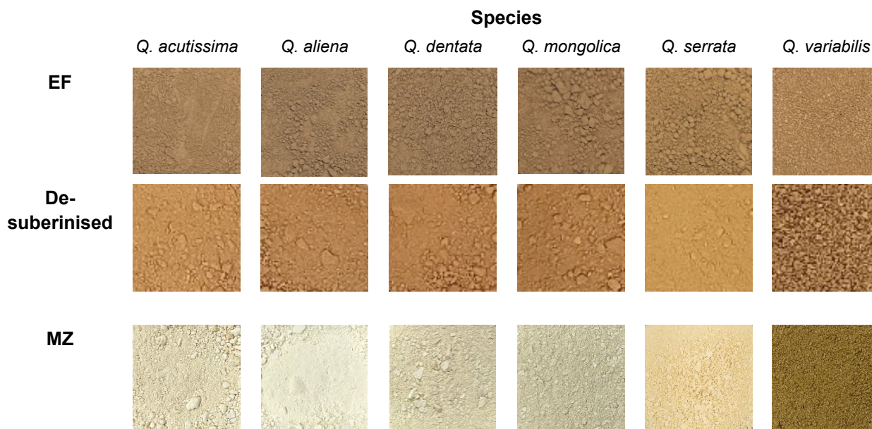
Fig. 2. Qualitative color results of extract-free (EF), de-suberinated material, and methanolizates (Desuberinised) of six Korean Quercus species (EF = methanolizates + lignin + carbohydrate; Desuberinised = lignin + carbohydrate; MZ = potential suberin-containing extract)
