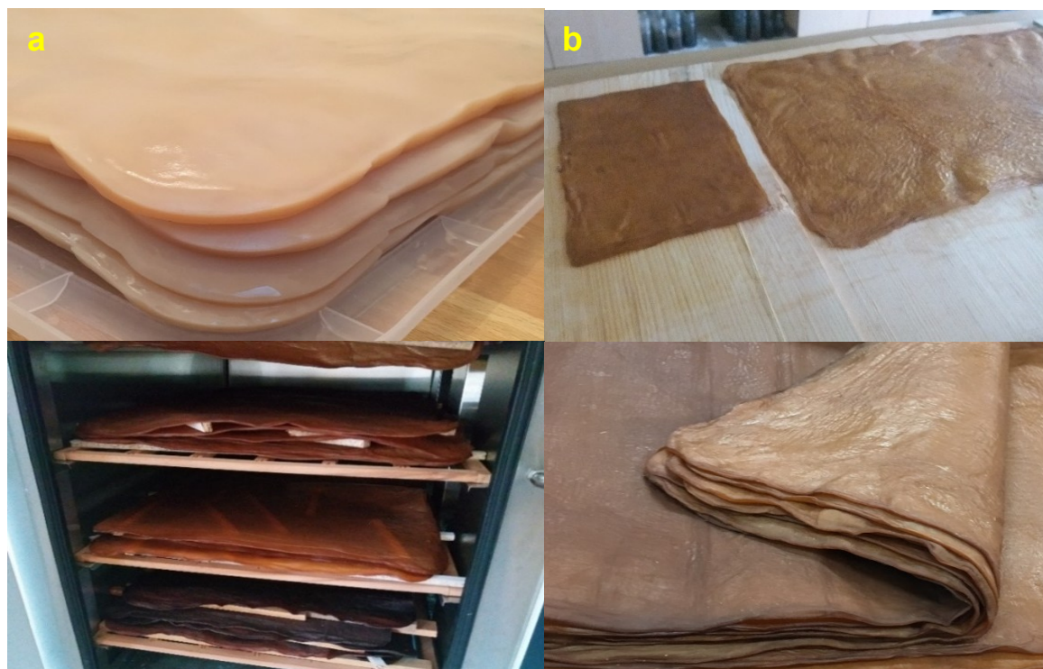
Fig. 1. Kombucha-derived BC pellicles: (a) conditioning/drying process; (b) stacked dried pellicles
