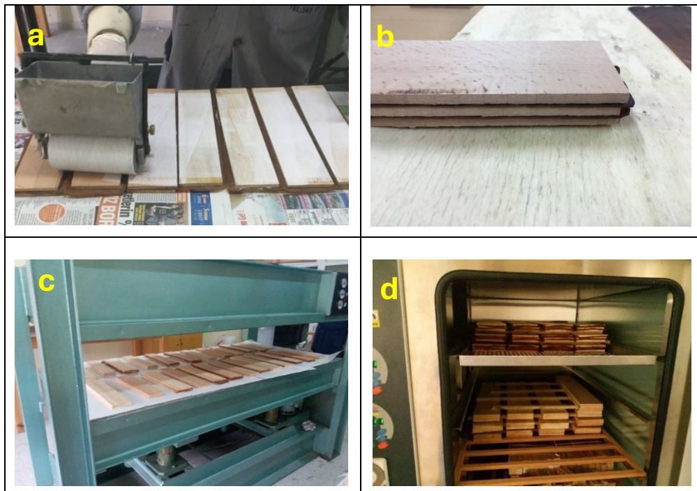
Fig. 3. Production process of laminated wood materials reinforced with BC sheets: (a) gluing, (b) layering, (c) pressing, and (d) conditioning
