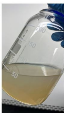
Synthesized Coating Solution of Cellulose/PVDF
