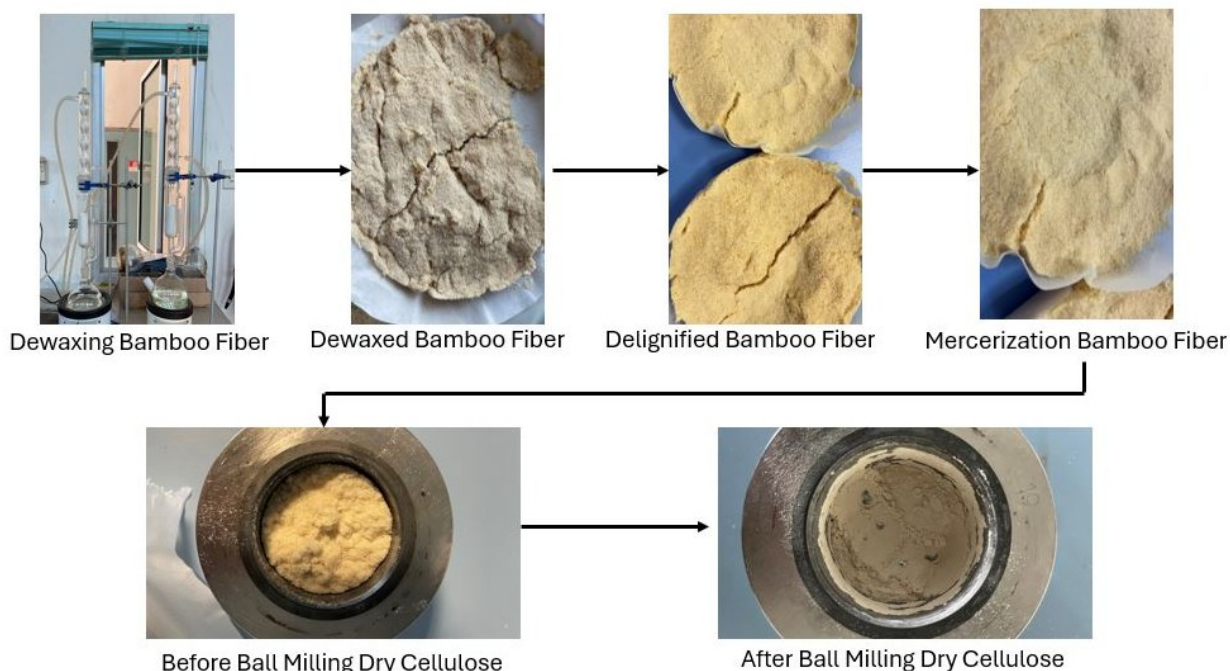
Fig. 1. Illustration of the extraction of bamboo cellulose from bamboo fiber.
