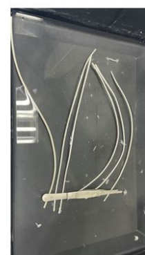
Phase Inversion water bath technique for all Coated PVDF hollow fiber membrane
