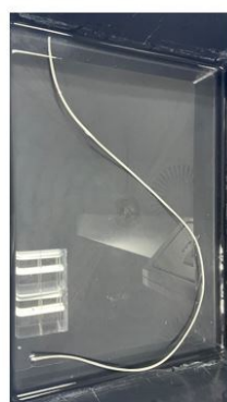
Phase Inversion water bath technique for all Coated PVDF hollow fiber membrane
