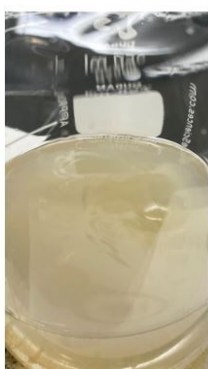
Synthesized Coating Solution of Cellulose/PVDF
