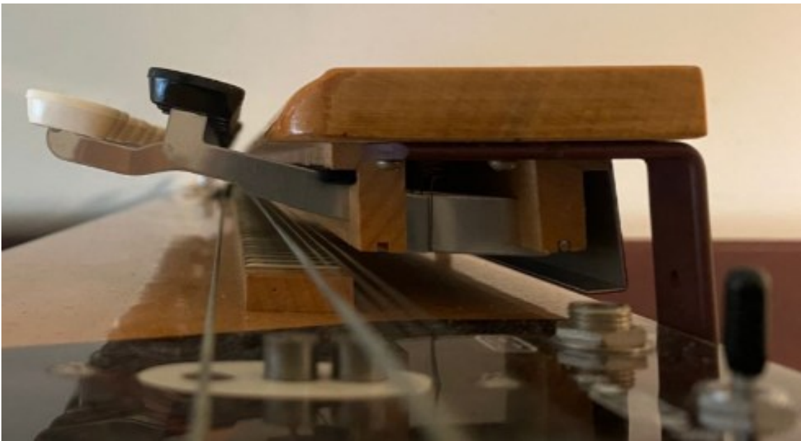
Fig. 3. The mechanism of contacting and holding the strings
